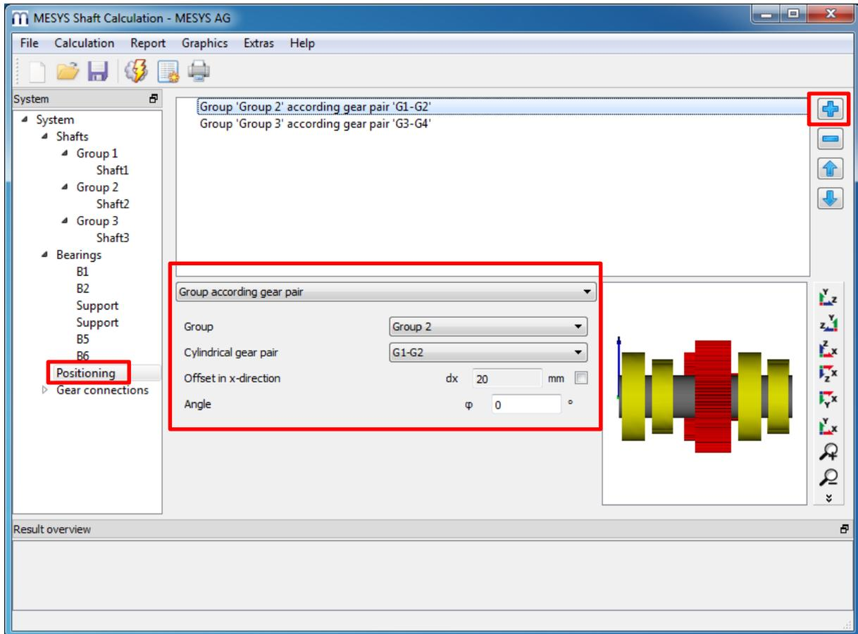
Add two constraints using the **+**-button on the right. Several options for positioning are available. Select 'Group according gear pair' and position 'Group2' with pair 'G1-G2' and 'Group3' with pair 'G3-G4'. The angle could be changed, we just leave it to 0° for this example, getting a vertical orientation of all shafts.
