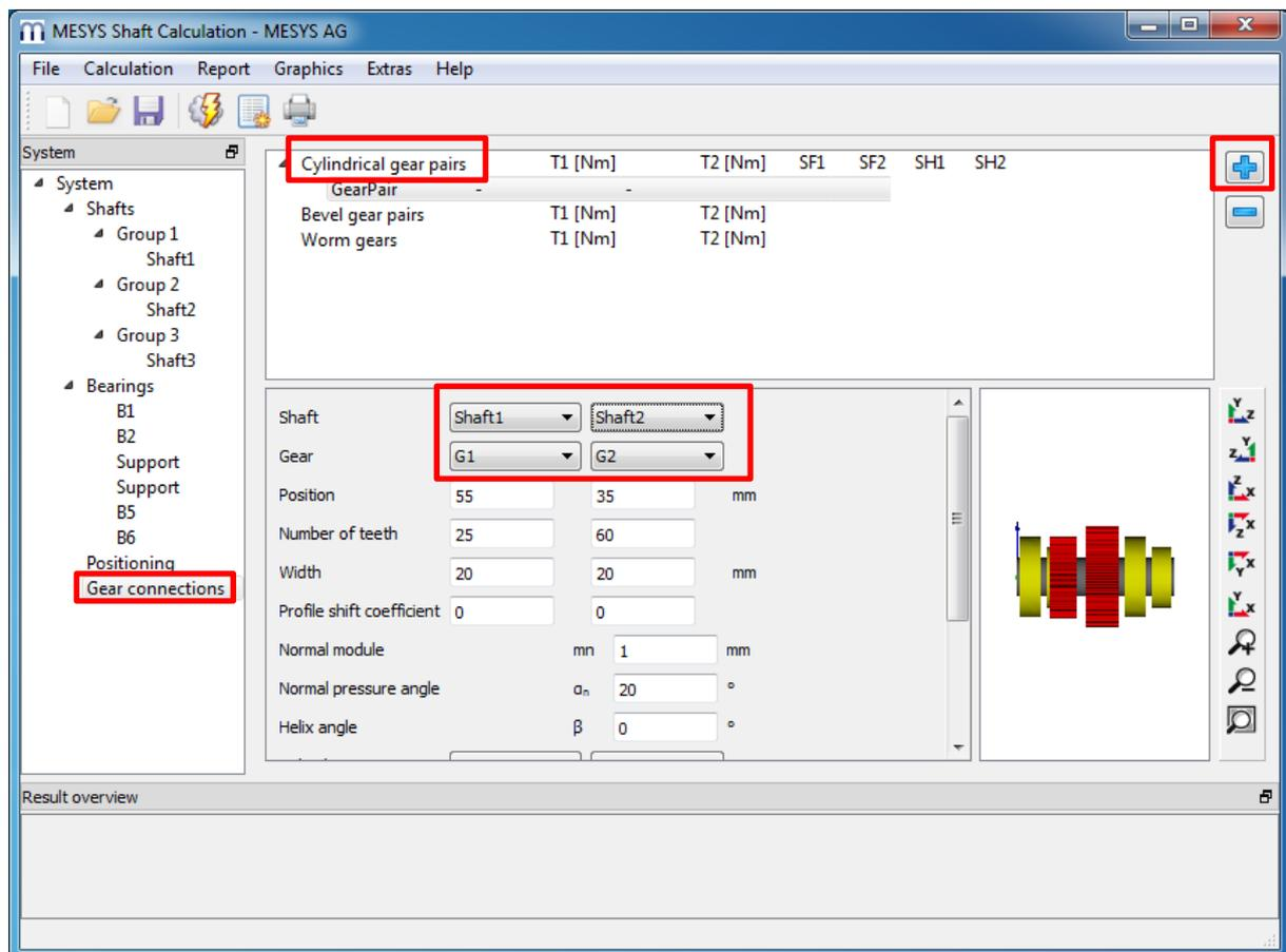
Now select the shafts and gears which should be connected. Connect G1-G2 for the first pair, then add a second pair and connect G3-G4. Circumferential backlash and gear mesh stiffness can be changed here. It is not needed to enter the center distance as it will be calculated later. The calculation program for the gear strength calculation can be selected if available.
