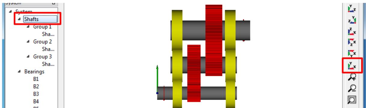
We see that there are collisions between the bearings. We go back to 'Gear connections' and change module for pair 'G1-G2' to 1.25 and to 1.75 for 'G3-G4'. Afterwards the space between the bearings is small, but we don't have any collisions:
