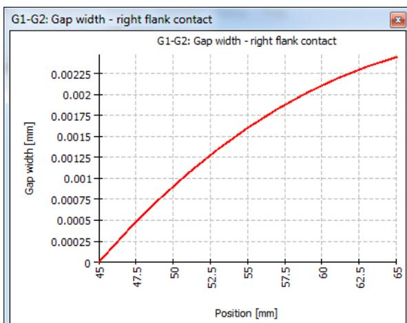
The gap width shows the gap between the flank if the contact would be just on one point. So in this case a flank line correction of  $2\mu\text{m}$  could be made. These diagrams are made with the setting 'Consider gears as stiffness' set. Gear mesh stiffness, shaft and bearing stiffness have an influence to these diagrams. But also manufacturing errors and housing stiffness have an influence on the real gearbox.
