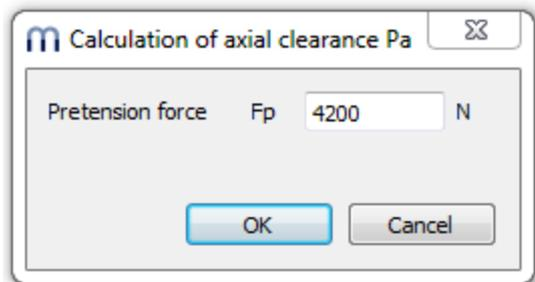
To get a pretension of 4.2kN we need an axial clearance  $P_a = -0.0525\text{mm}$ .
