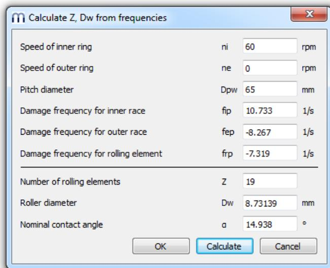
Note that  $D_w$  and  $\alpha$  must be manually rounded off on the page "Bearing geometry" so that they match standard values (The calculated  $D_w$  is practically equal to an usual one with  $11/32$  inch = 8.731mm, and the contact angle to  $15^\circ$ ).
