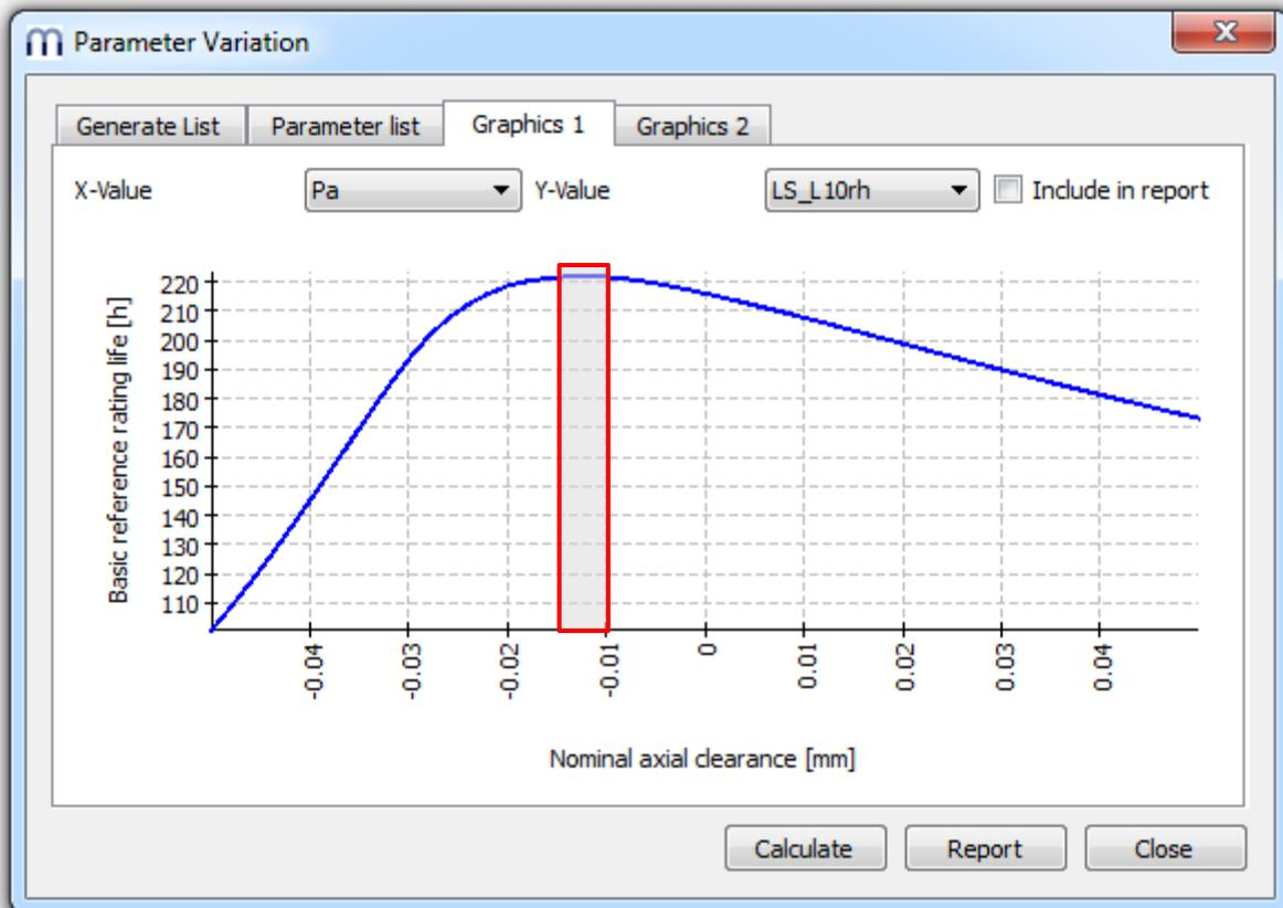
Please note that for each load case, a full calculation using all factors is made. The resulting life is calculated using the life of each element.
