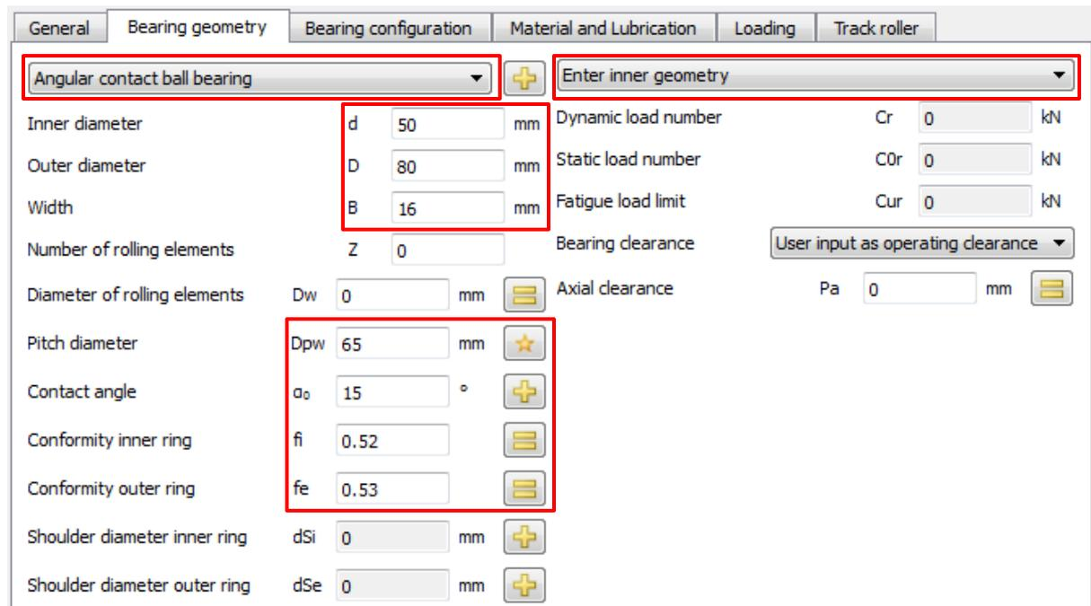
Since the conformity is not provided we use the values according to ISO/TS 16281 with  $f_i = 0.52$  and  $f_e = 0.53$
