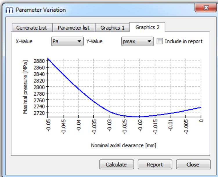
For instance, in case we assume that the bearing must have a certain pretension, the user can deduce from this study, that the higher the pretension is, the shorter life the bearing has. However, if we widen the range of the possible axial clearances to the positive direction of X-Value for the bearing, we can identify a maximum over the range  $P_a = (-0.01, 0)$  mm:
