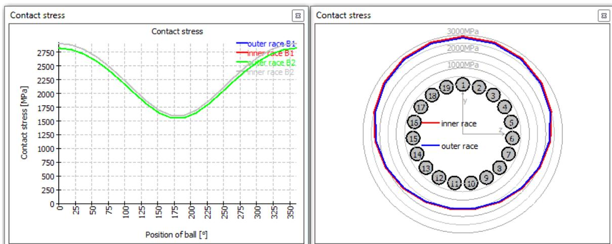
When performing the calculation according ISO 281 without pretension, we get a result of  $L_{10h} = 16666/2200 * (28.2 * 2^{0.7}/15)^3 = 215h$  instead of the  $L_{10h} = 87h$  with pretension by the software.
