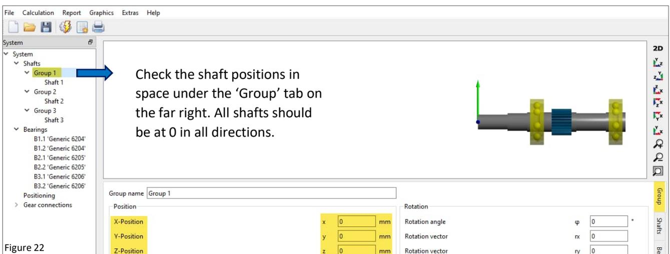
Check the shaft positions in space under the 'Group' tab on the far right. All shafts should be at 0 in all directions.
