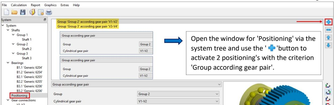
➡ Open the window for 'Positioning' via the system tree and use the '+' button to activate 2 positioning's with the criterion 'Group according gear pair'.
