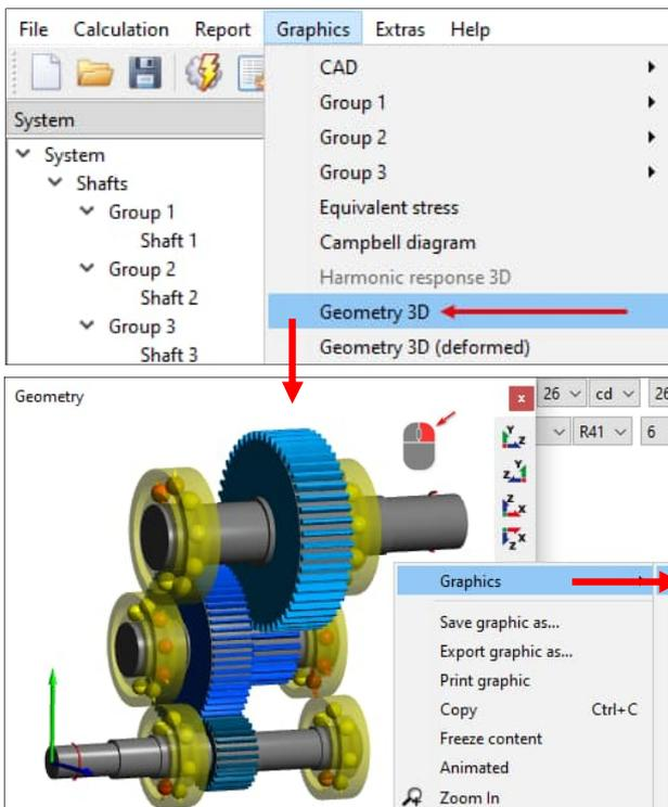
Through the context menu and by selecting the 3D Geometry option, the shaft system or its components can be exported as an STL or STEP file for further use:
