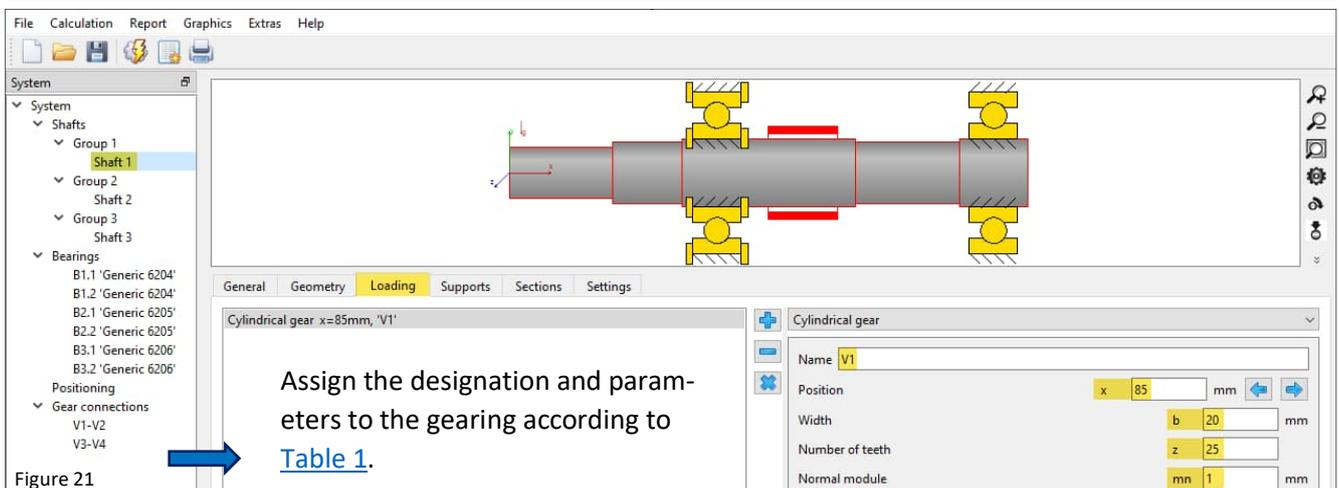
Assign the designation and parameters to the gearing according to [Table 1](#).
